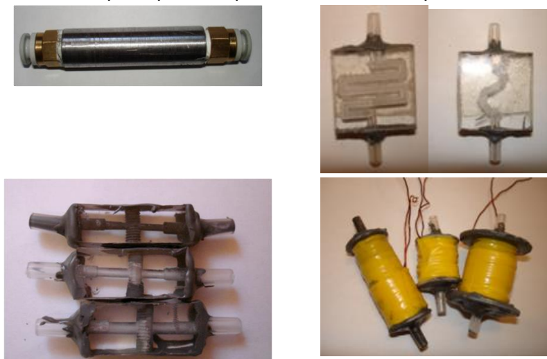
Figura 1.5. Modele constructive valve-stop magnetoreologice
